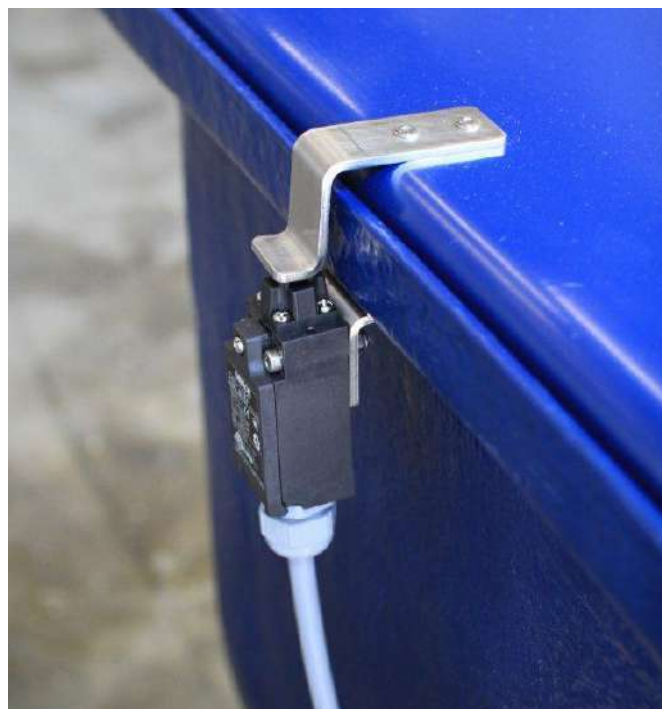
Safety switch stops the drum when the lid is opened.
